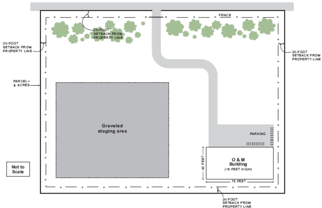
Figure 3-1: Typical O&M Facility Layout
